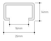
Tecties 25/14 channel features alternate 6mm and 8mm diameter holes to accept different fixings.
