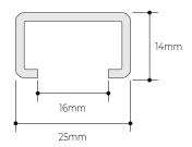
Tecties 25/14 channel features alternate 5.3mm and 9.5mm diameter holes to accept different fixings.
