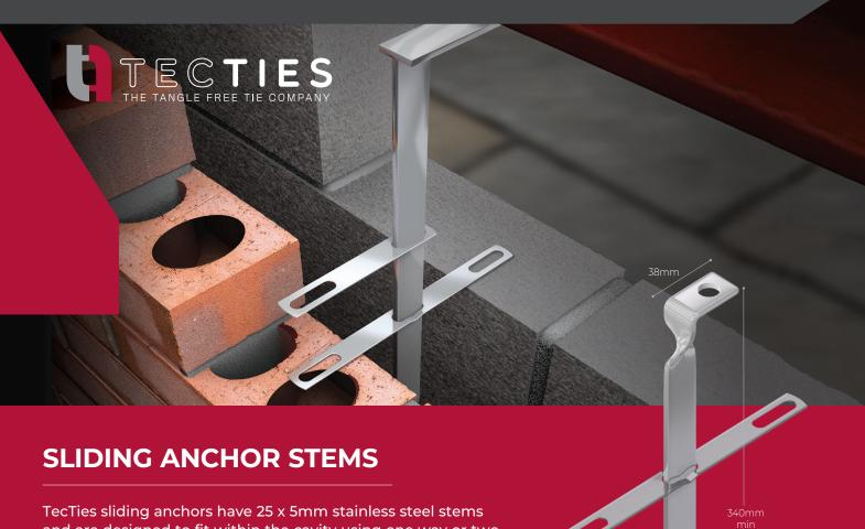
TecTies sliding anchors have 25 x 5mm stainless steel stems and are designed to fit within the cavity using one way or two way safety ties, that slide to accommodate vertical movement when restraining cavity walls to overhead structures.
